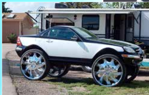
Spotted this 'DONK' cruising our campground in Colorado Springs. 2002 Mercedes SLK, 32 inch wheels, 3.5L Mercedes with a Ford C4 Trans, Suzuki Samurai front axle, Ford F150 narrowed rear. The owner is Roy Spiker, retired business owner in Lakeland, FL. He must have gotten bored or something.
