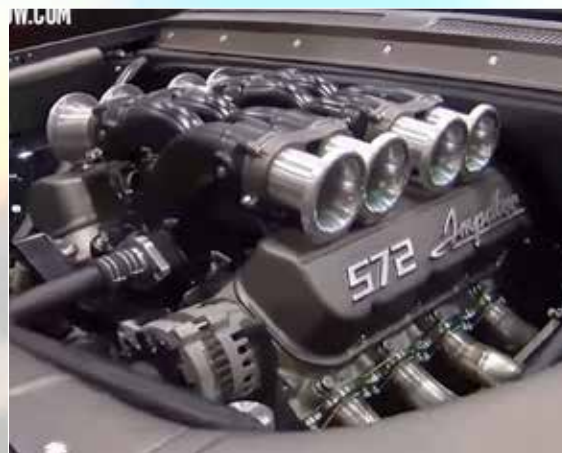
"The Impaler" – 1961 Chevrolet Impala Post Sedan with an eight stack injected 572 Chevy. I met Brian Fuller and saw this build at a Dover Speedway show ten years ago, but I could not find my photos of it. Here it is at SEMA.
